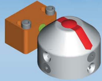
NAMUR VDI/VDE3845 connection to limit switches
